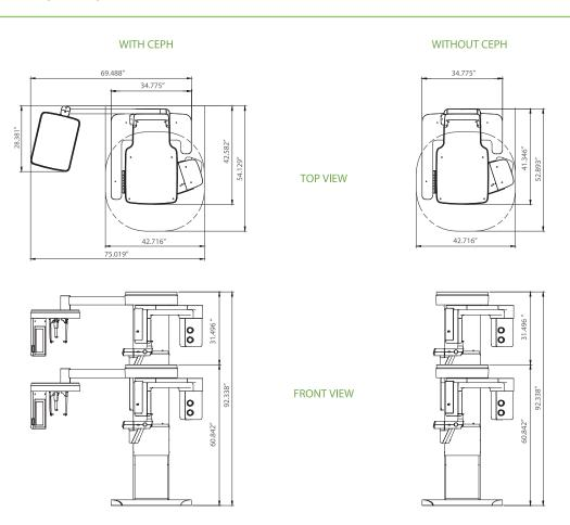
\*An additional 3 inches (76.2 mm) of space is required behind the unit for wall mount bracket installation (mandatory unless there is a base mount installation).
